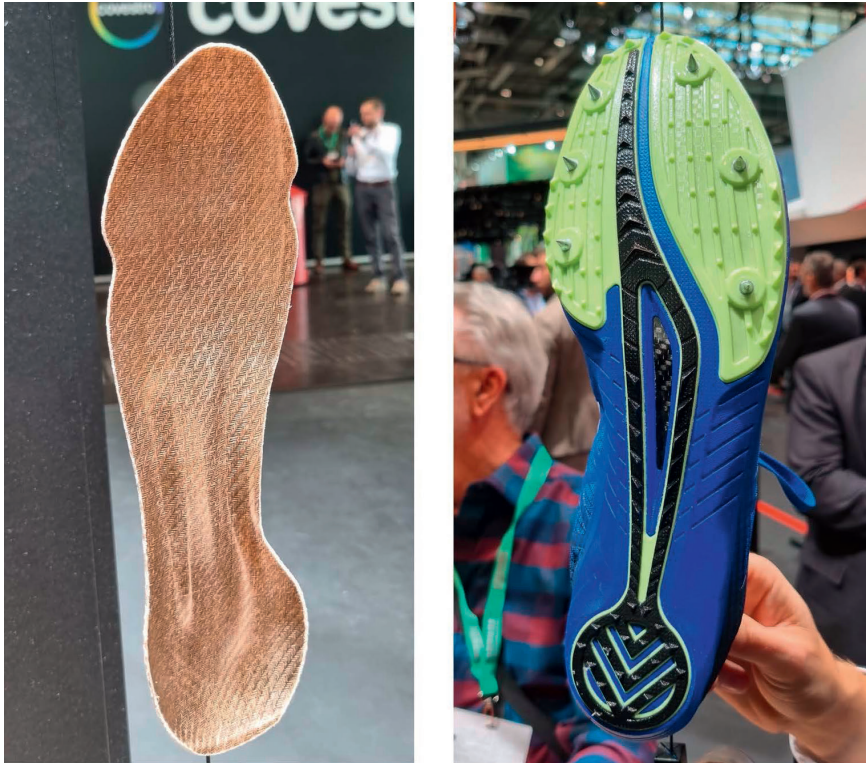
Fig. 3. As an alternative for conventional fiber-reinforced materials (right) for shoe soles, Lanxess has developed a completely bio-based TepeX (left). Consisting of PLA, it is reinforced with flax fibers. © Hanser/F. Streifinger
