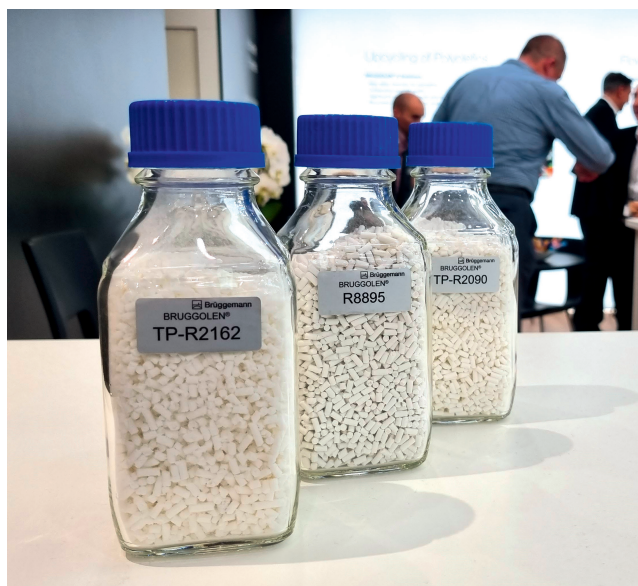
Fig. 5. Normally, recyclates must be re-stabilized with additives during the recycling process. Three newly introduced additive types enable the quality of PE and PP to be increased significantly.
